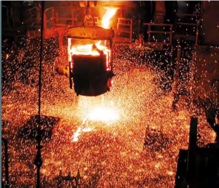
1_ Molten metal is decanted from an electric arc oven
